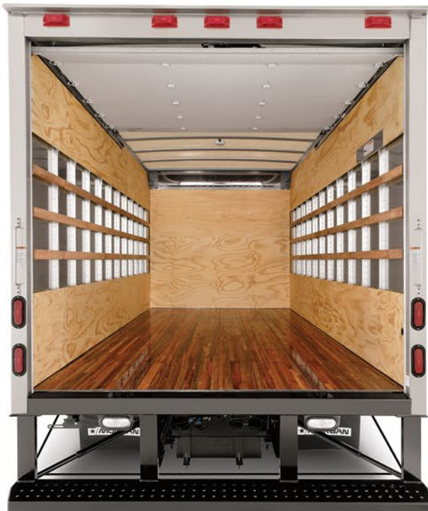
Cargo Interior - Plywood and Tie Slats, Floor Varnish
