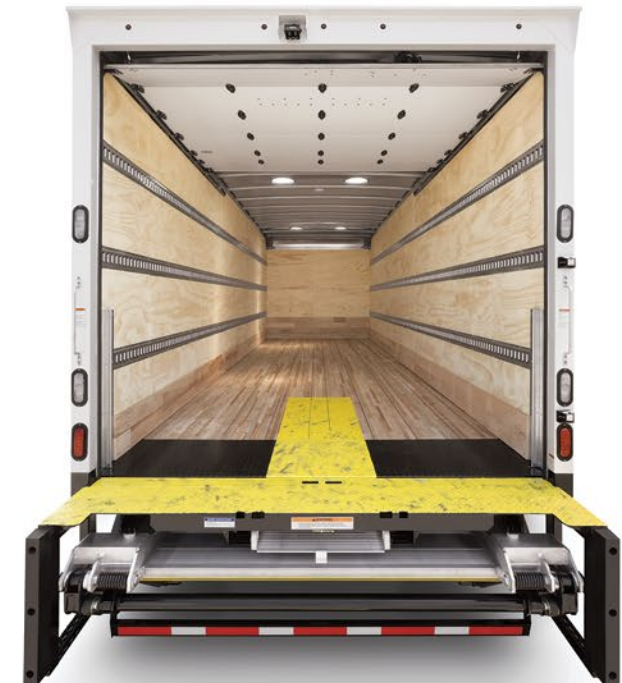
Cargo Interior - Plywood and E-track, Sky-Lights in Roof
