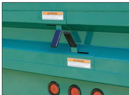
Lever activated dual-action gate
