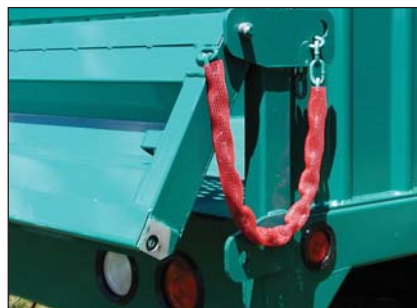
Gate in spreader mode
