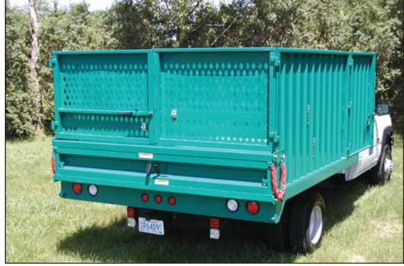
2-piece perforated upper rear doors
